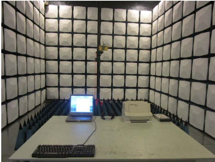
Radiated Emission Above 1GHz –Front View
