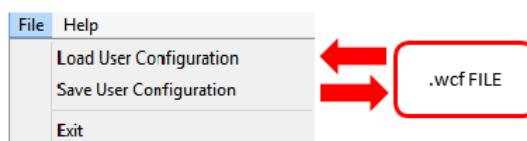
Using a file menu at the top left of the panel it is possible to **load/save all the configuration** values of the device to/from a .wcf file (Wisicom Configuration File).
