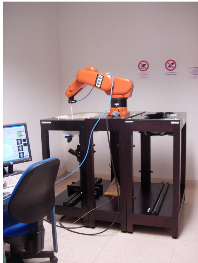
Picture A - SAR Dosimetric Assessment System
