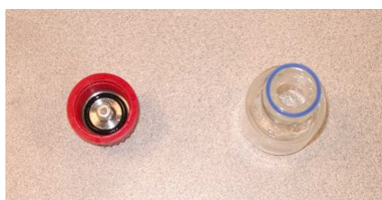
Picture E: open coaxial probe with the bottle cap
