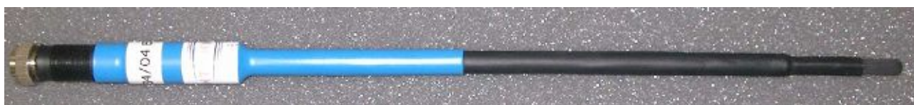
Picture D – isotropic E-Field Probe
