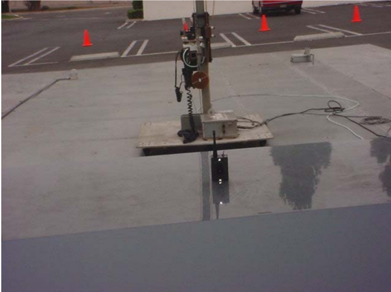
Field Strength emission measurements (15.109 / 209, 15.249a) View 2
