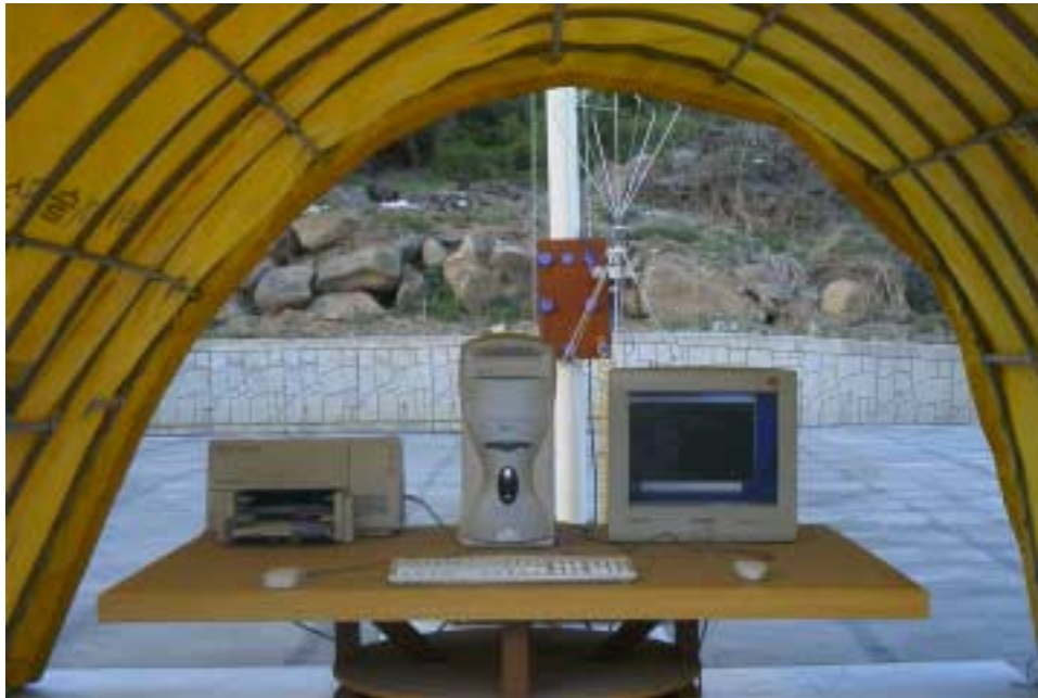
Photograph 1 : Setup for radiated Emissions
