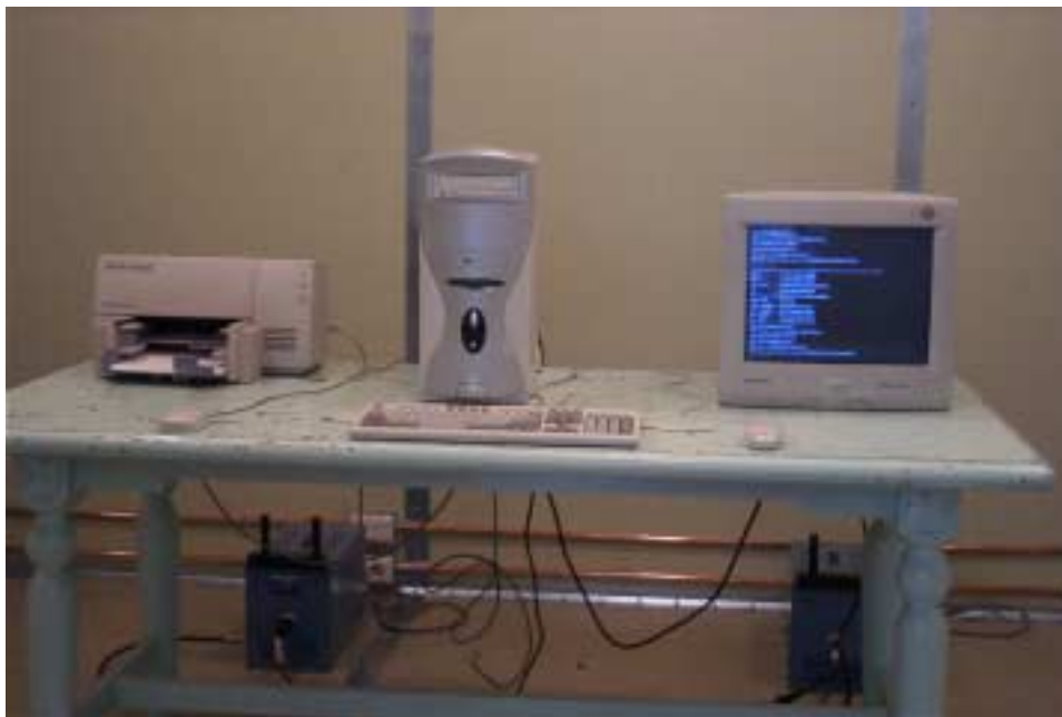
Photograph 2 : Setup for Conducted Emissions
