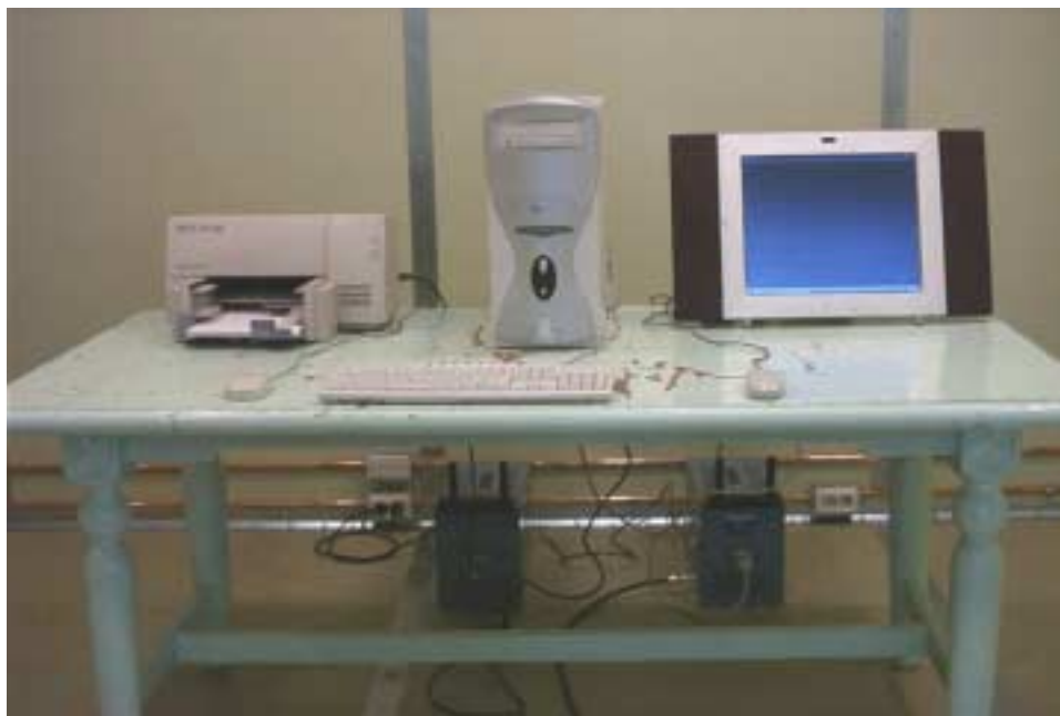
Photograph 2 : Setup for Conducted Emissions
