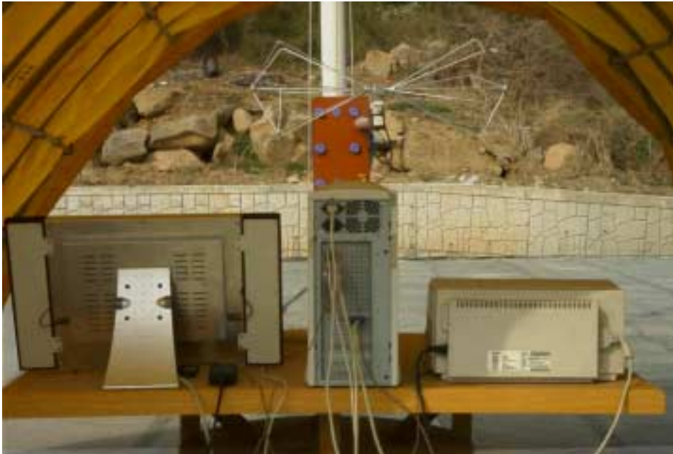
Photograph 1 : Setup for radiated Emissions
