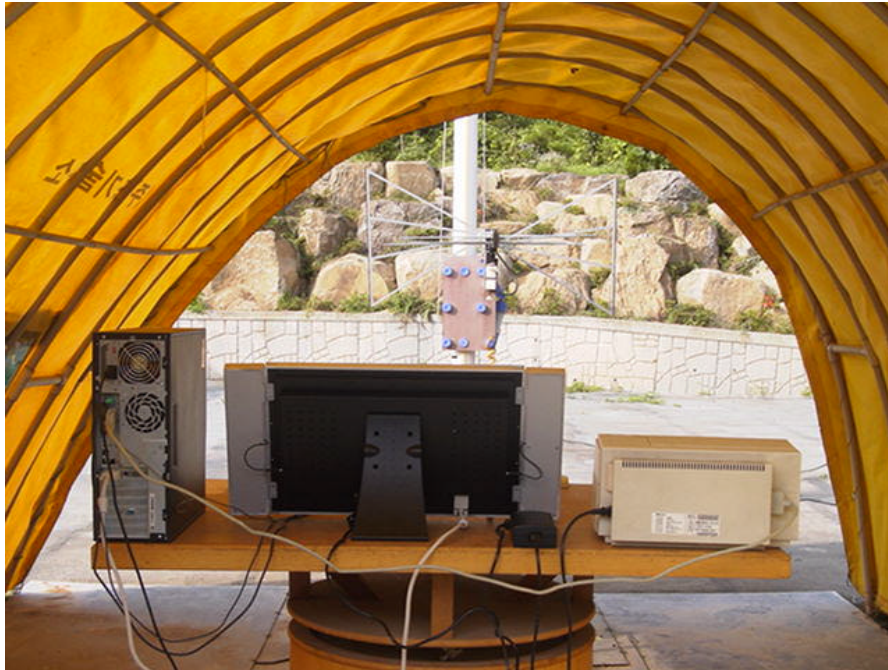
Photograph 1 : Setup for radiated Emissions
