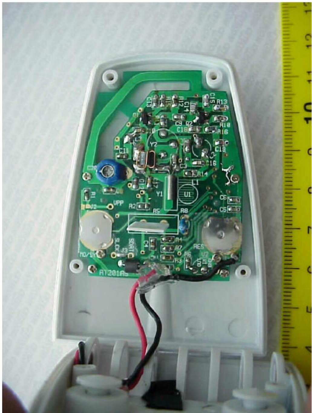
**Photographs of the equipment: Transmitter WS260**
