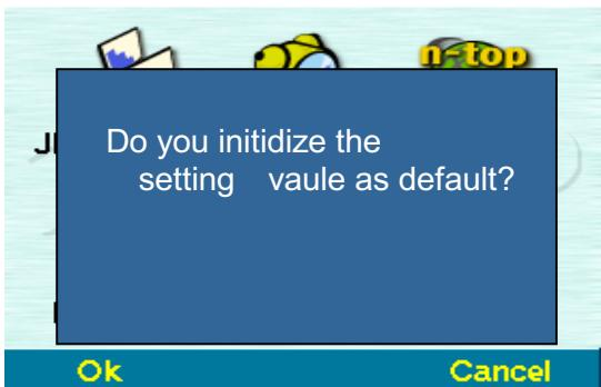
If pressing the enter button, the environmental setup values go back to the initial condition and return to the initial screen.
