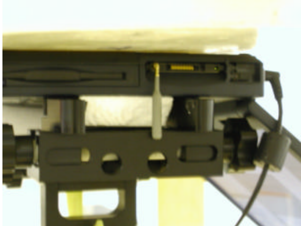
Photo 2: HP T18.033.C.00 Bottom of laptop flush with phantom, antenna parallel to laptop side and perpendicular to phantom
