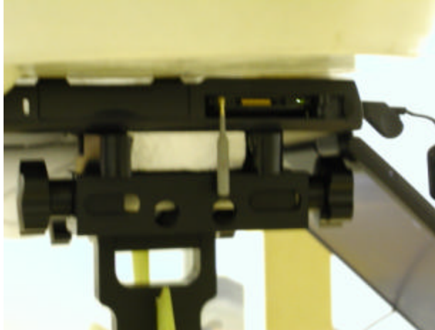
Photo 7: Dell PP01L Bottom of laptop flush with phantom, antenna parallel to laptop side and perpendicular to phantom
