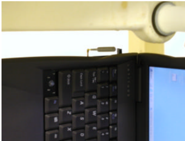
Photo 8: Dell PP01L bystander position with 1.5cm separation distance
