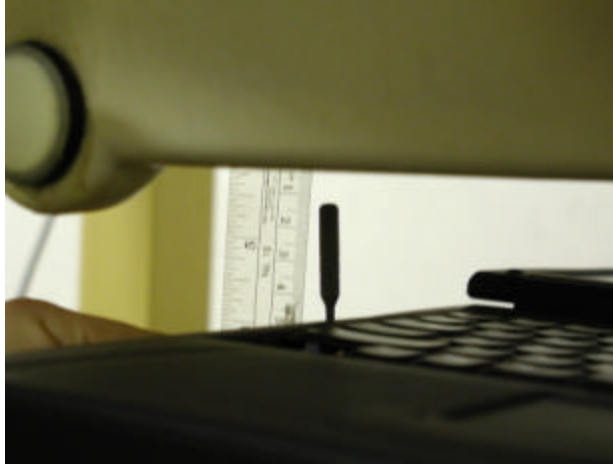
Photo 9: Dell PP01L keyboard facing with phantom, antenna perpendicular to laptop
