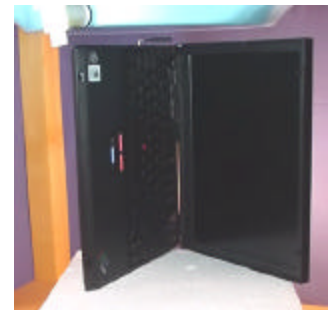
Body SAR Test Setup with 1.0cm separation distance
