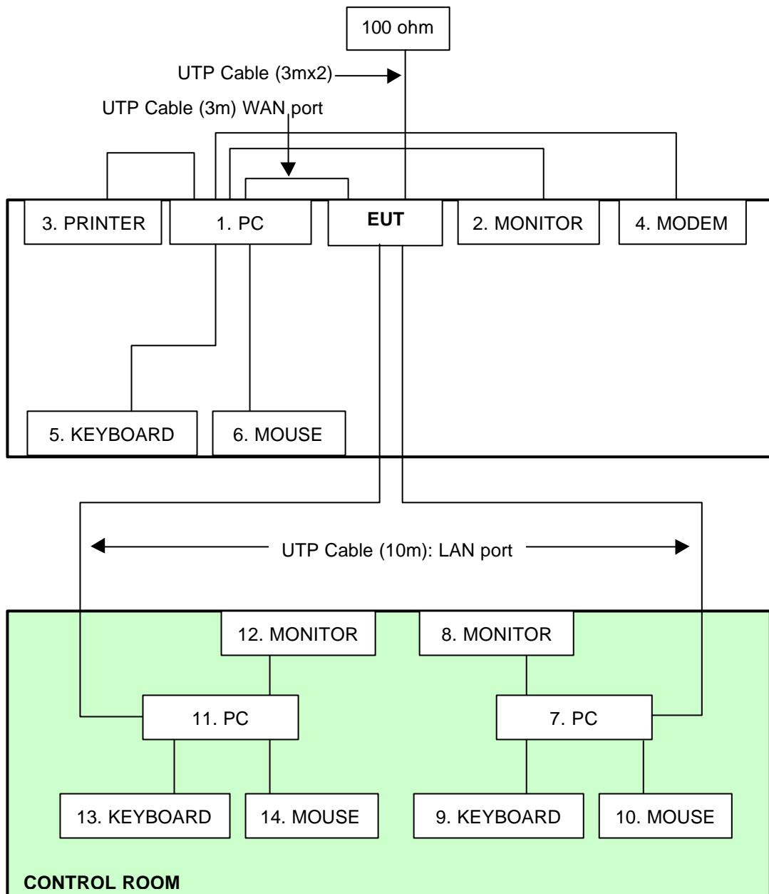
**NOTE:** 1. Support units 7-14 were kept in the control room during the test.
