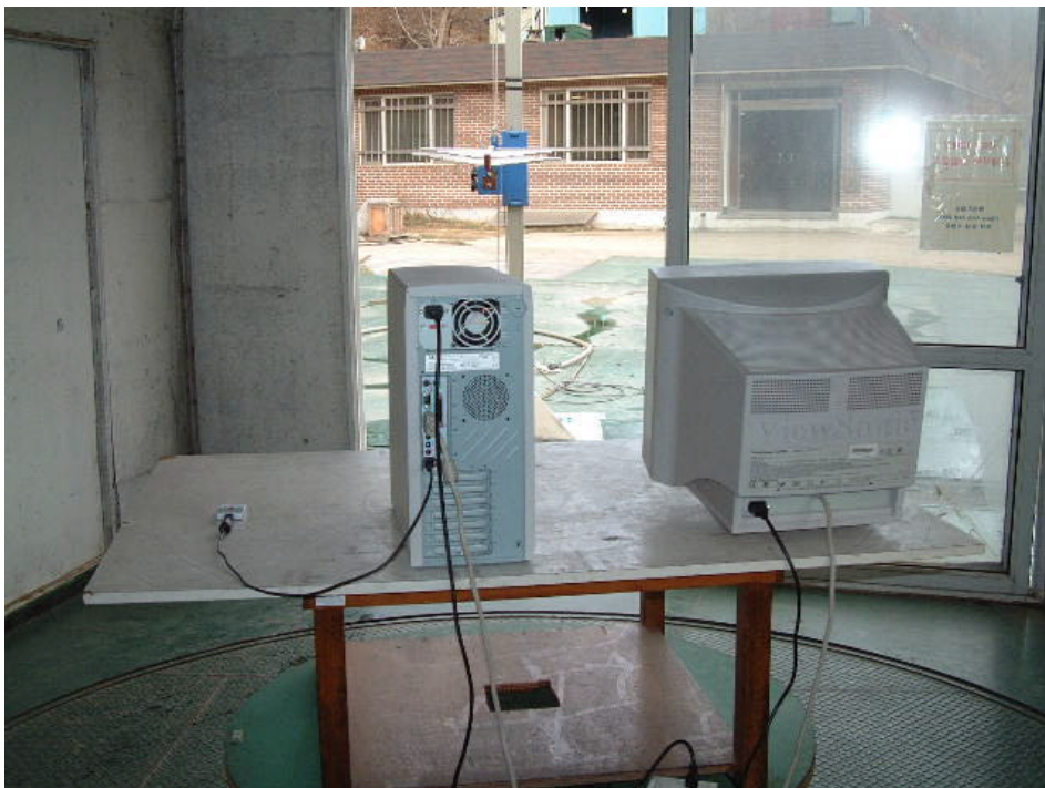
RADIATED EMISSION SETUP PHOTOGRAPH - REAR VIEW ( 300 - 1000 MHz )
