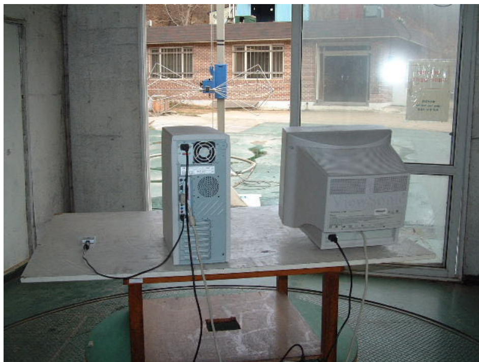
RADIATED EMISSION SETUP PHOTOGRAPH - REAR VIEW ( 30 - 300 MHz )
