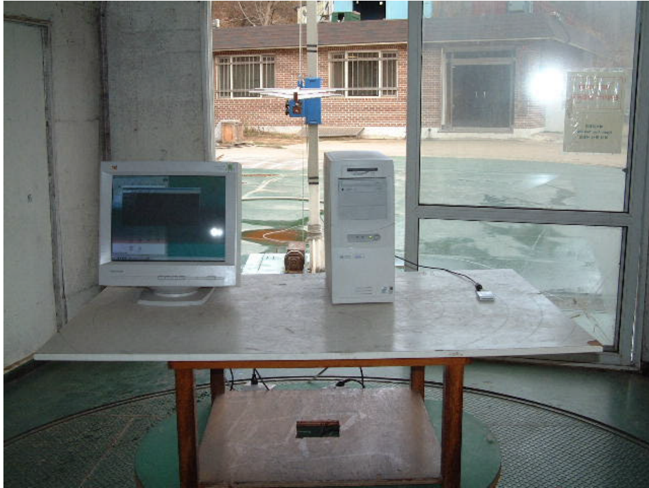
RADIATED EMISSION SETUP PHOTOGRAPH - FRONT VIEW ( 300- 1000 MHz )
