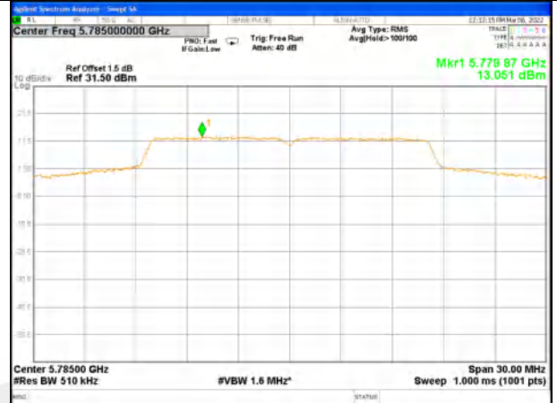
W58_11n20_Lower_Power Spectrum Density
