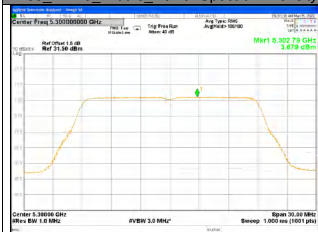
W53_11n20_Middle_Power Spectrum Density
