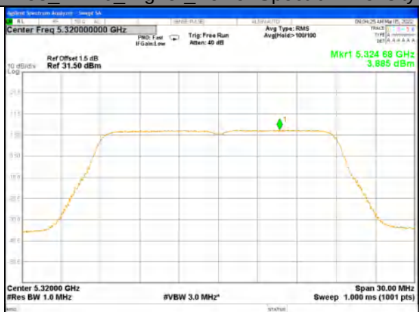
W53_11n20_Higher_Power Spectrum Density
