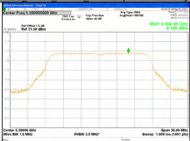
W53_11n20_Lower_Power Spectrum Density
