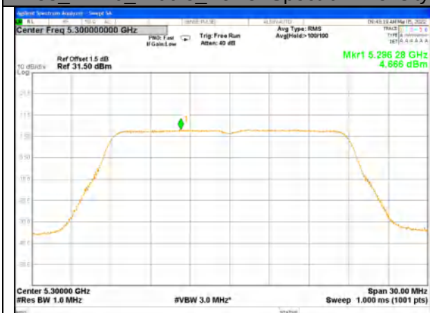
W53_11n20_Middle_Power Spectrum Density
