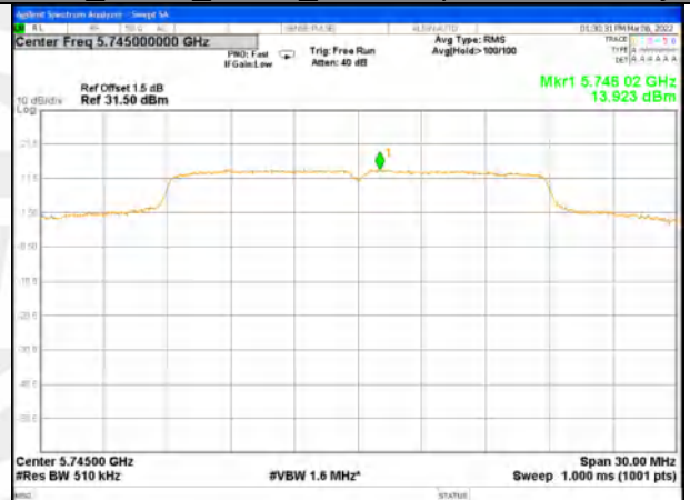
W58_11n20_Higher_Power Spectrum Density
