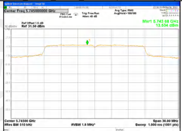
W58_11n20_Higher_Power Spectrum Density
