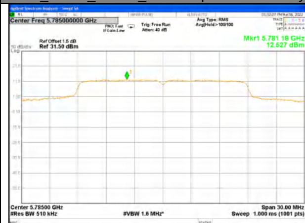
W58_11n20_Middle_Power Spectrum Density
