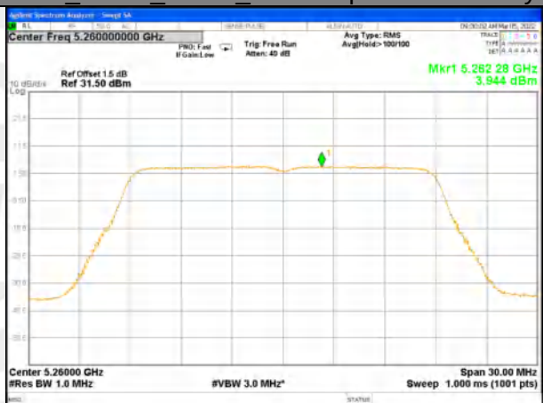
W53_11n20_Higher_Power Spectrum Density
