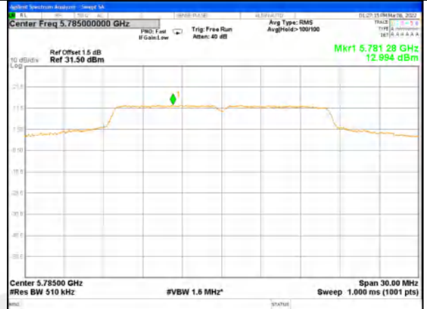
W58_11n20_Lower_Power Spectrum Density
