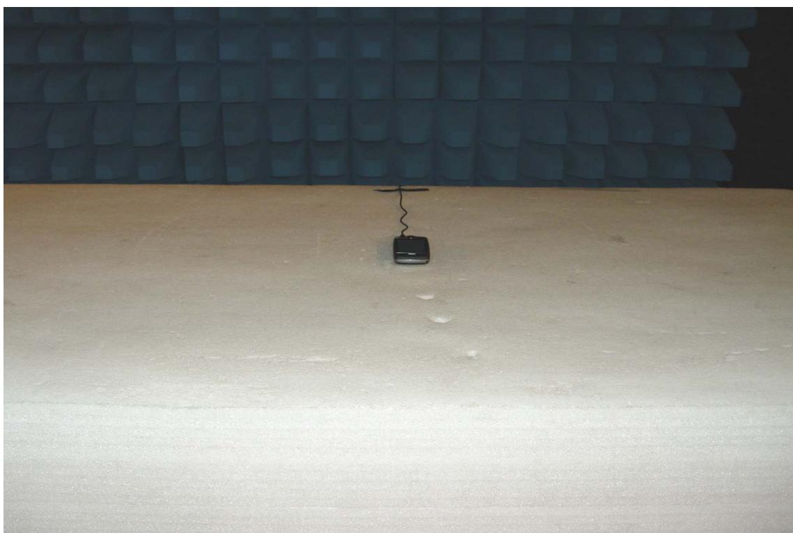
**POWERLINE CONDUCTED EMISSIONS SETUP PHOTOS**
