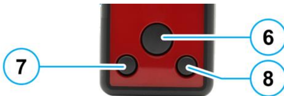
Fig. 4: Hardware reset: Press button no. 7 and 8
