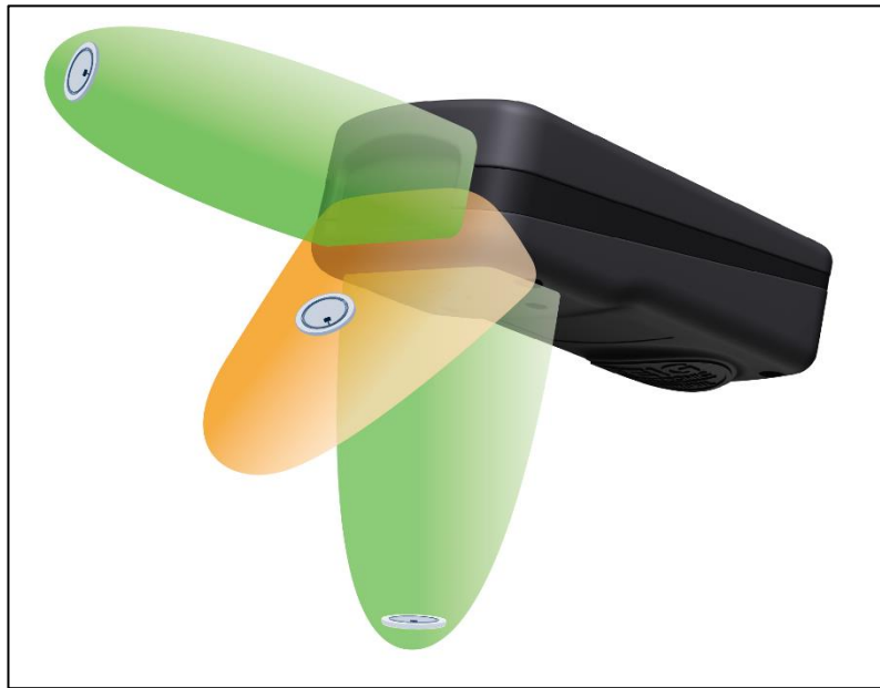
Fig. 5: RFID detection areas (bottom & front) of the reader
