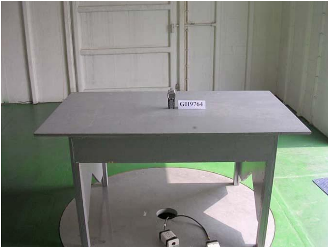
Photo 4: Radiated Emission Test Set-up (Handset)
