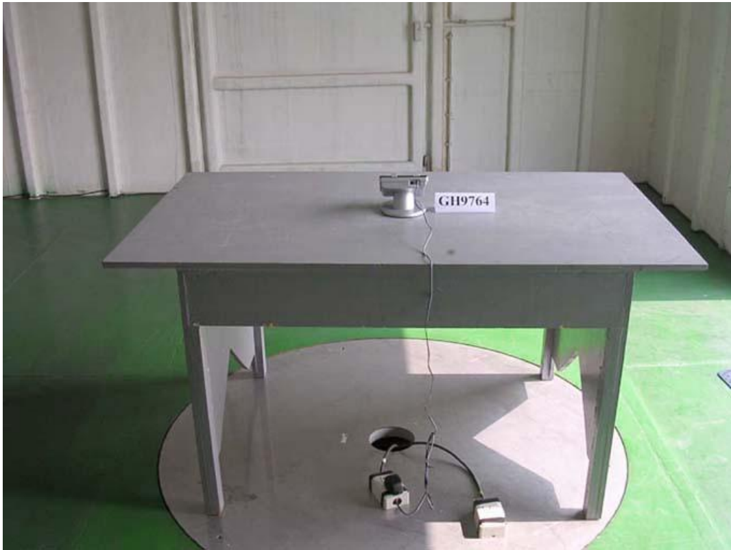
Photo 3: Radiated Emission Test Set-up (Base)
