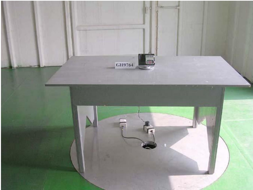
Photo 1: Radiated Emission Test Set-up (Base)
