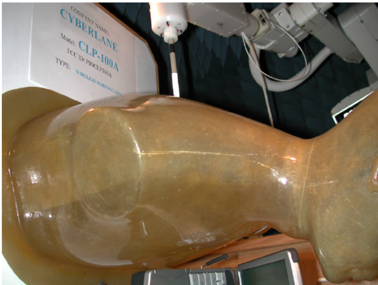
Fig 8. Test Setup of EUT in operating position with the source of significant emissions (antenna) 1.5 cm below the phantom.
