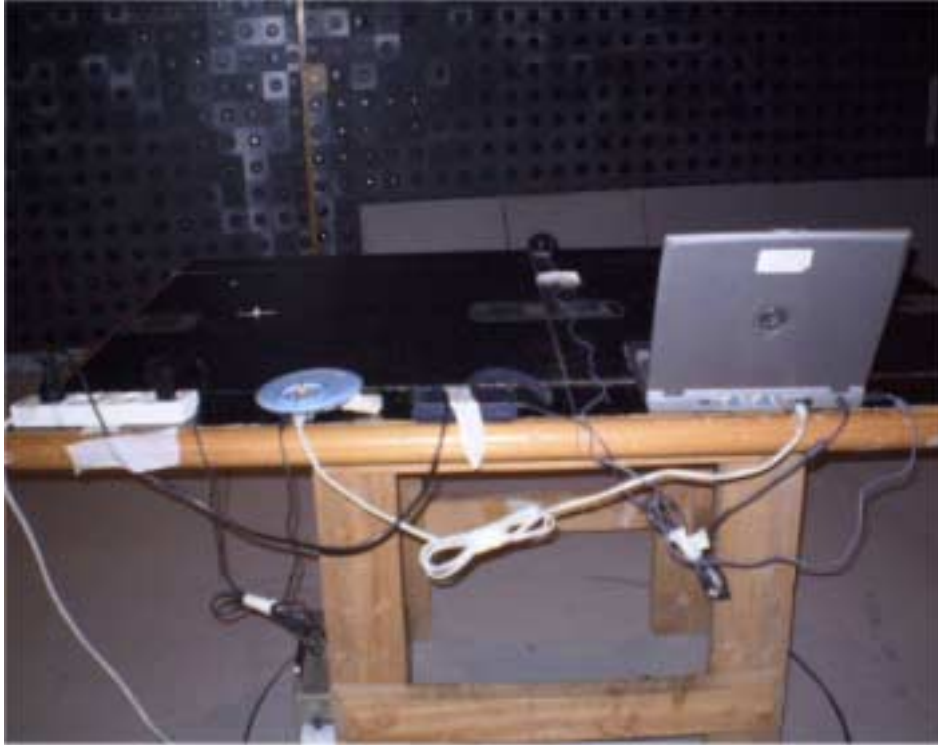
Photograph No.6 Radiated emissions measurement setup in the anechoic chamber, close view
