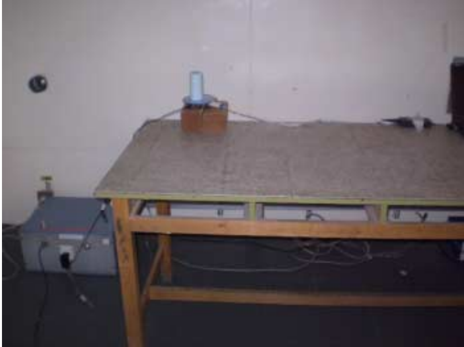
Photograph No.9 Conducted emissions measurement on AC line setup
