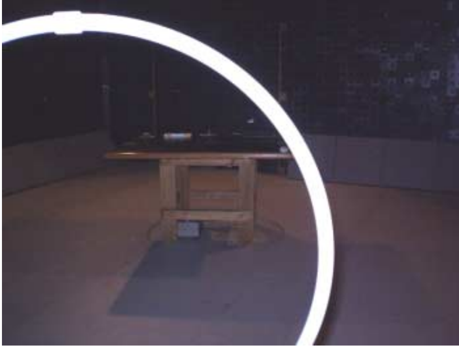
Photograph No.3 Radiated emissions measurement setup in the anechoic chamber below 30 MHz
