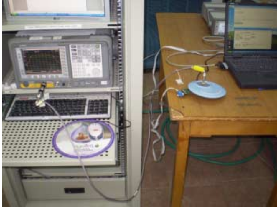
Photograph No.2 Power spectral density, occupied bandwidth, conducted spurious emissions measurement setup
