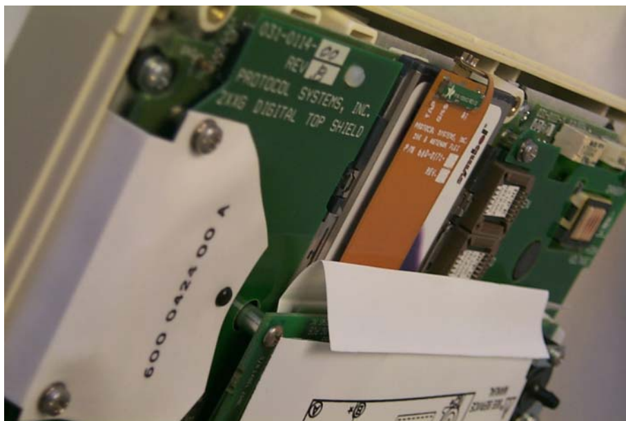
EUT with Antenna installed in PC Card Slot inside of Host Unit
