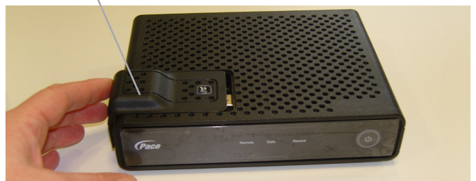
Push adapter gently but firmly into position.
