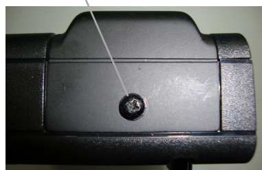
Philips-head fixing screw on WiFi adapter
