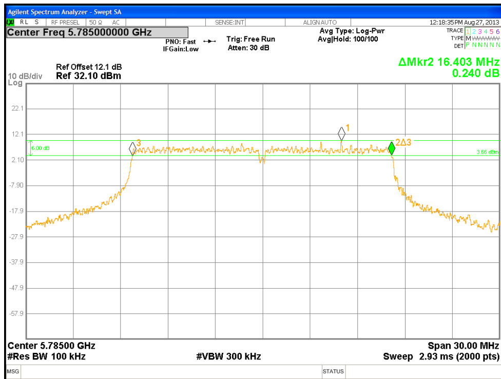
Figure 47: DTS Bandwidth at 5785 MHz, 802.11A, Chain 3
