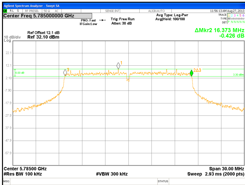
Figure 41: DTS Bandwidth at 5785 MHz, 802.11A, Chain 0
