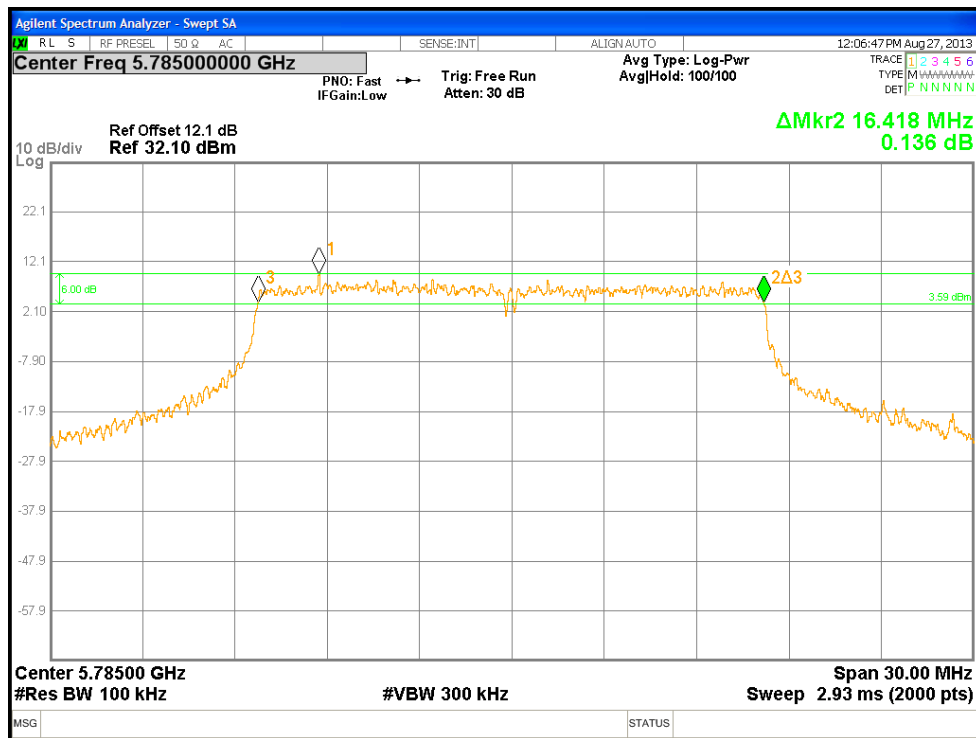
Figure 43: DTS Bandwidth at 5785 MHz, 802.11A, Chain 1
