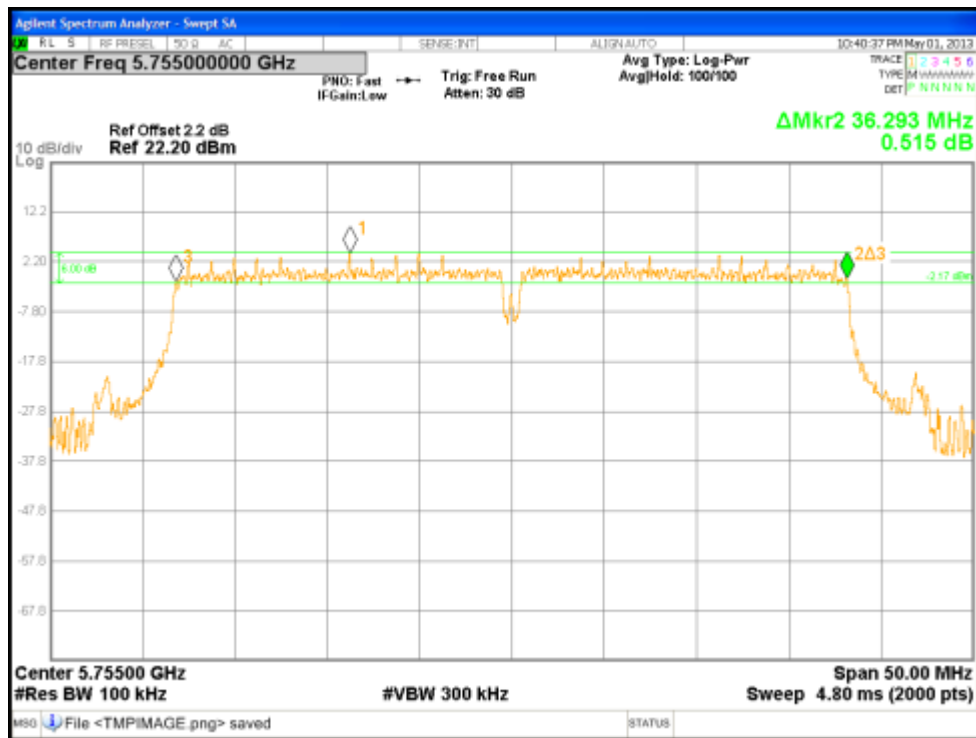
Figure 87: DTS Bandwidth at 5755 MHz, Chain 3
