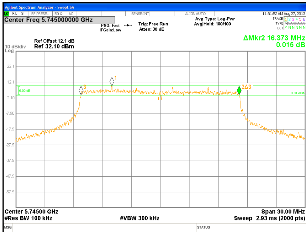
Figure 35: DTS Bandwidth at 5745 MHz, 802.11A, Chain 1
