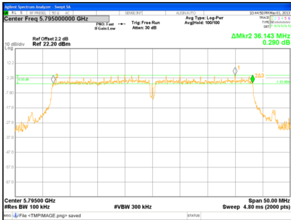
Figure 91: DTS Bandwidth at 5795 MHz, Chain 1
