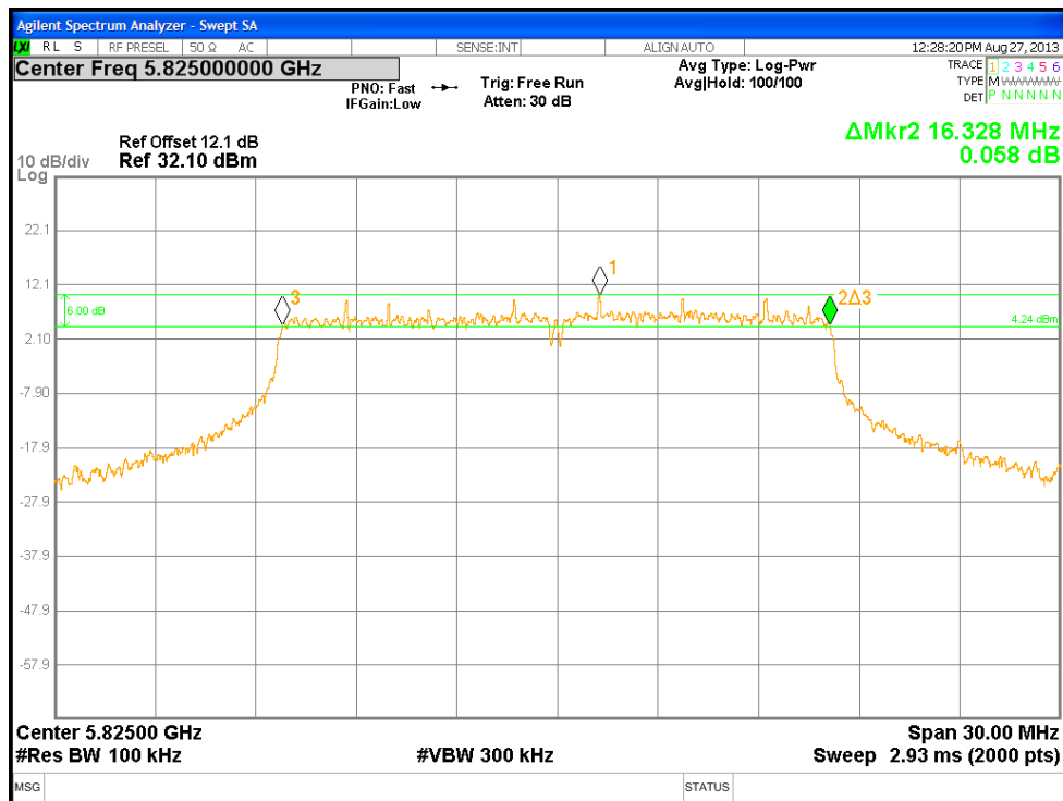
Figure 49: DTS Bandwidth at 5825 MHz, 802.11A, Chain 0
