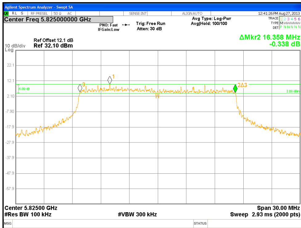
Figure 53: DTS Bandwidth at 5825 MHz, 802.11A, Chain 2
