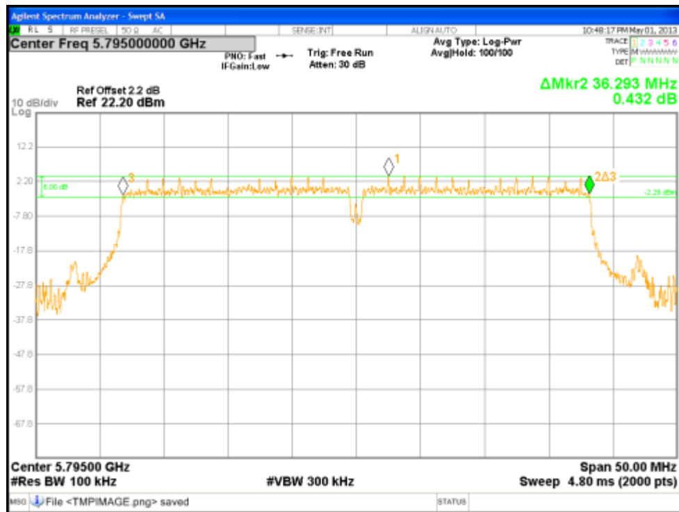
Figure 95: DTS Bandwidth at 5795 MHz, Chain 3
