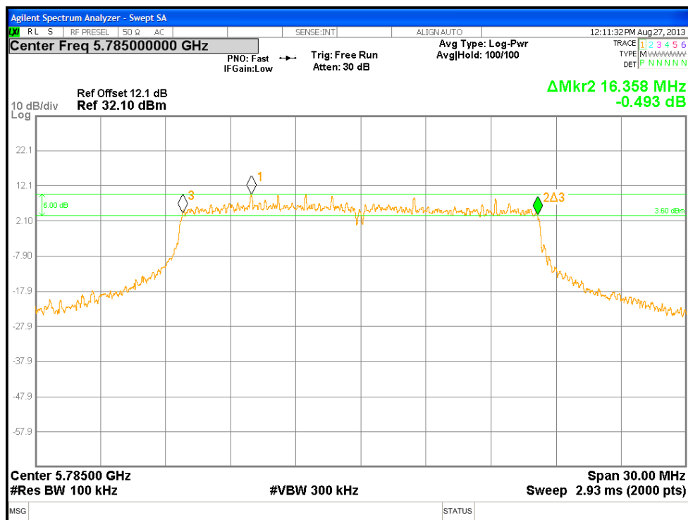
Figure 45: DTS Bandwidth at 5785 MHz, 802.11A, Chain 2
