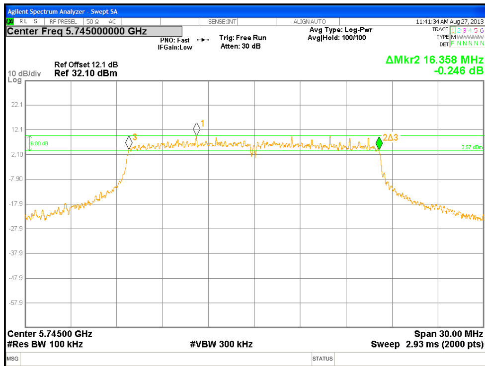
Figure 37: DTS Bandwidth at 5745 MHz, 802.11A, Chain 2
