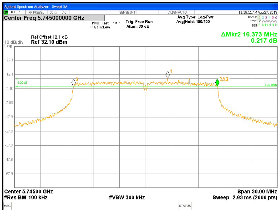
Figure 33: DTS Bandwidth at 5745 MHz, 802.11A, Chain 0
