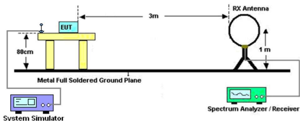
For radiated emissions from 30MHz to 1GHz
