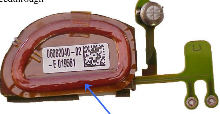
Orange coil is part of magnetically coupled communications system (not part of RF circuit).
