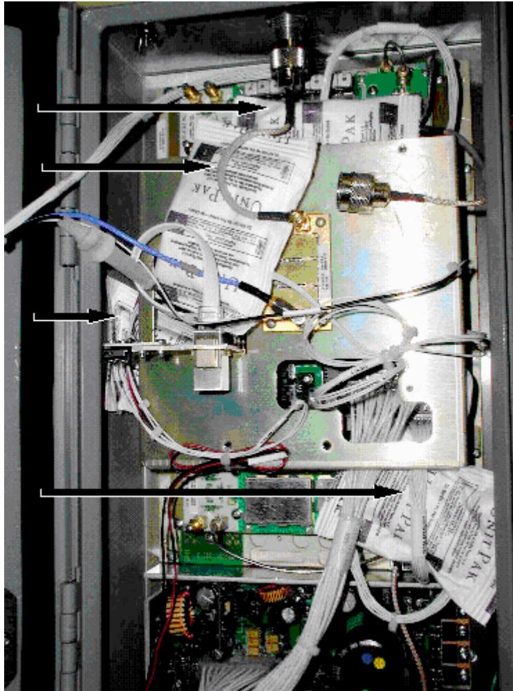
figure 21. cSPICE dessicant locations
