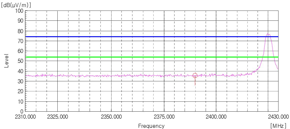
AV Detector: RBW: 1 MHz, VBW: 10 Hz (2 310 MHz - 2 390 MHz), Worst case (Low, Horizontal)
