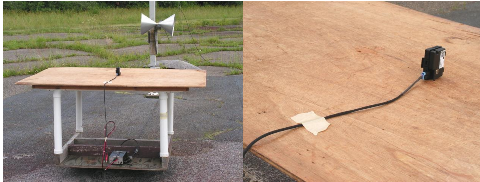
Figure 4: Radiated Emissions Test Setup Photograph(s).
