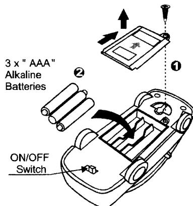
USE 3 X "AAA" SIZE (1.5V) ALKALINE BATTERIES WITH POLARITY AS SHOWN INSIDE BATTERY COMPARTMENT
