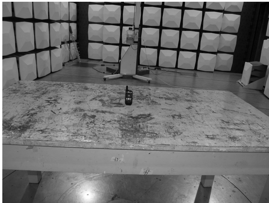
Photograph 3: Set-up for Spurious Radiation Emission Measurement below 1GHz
