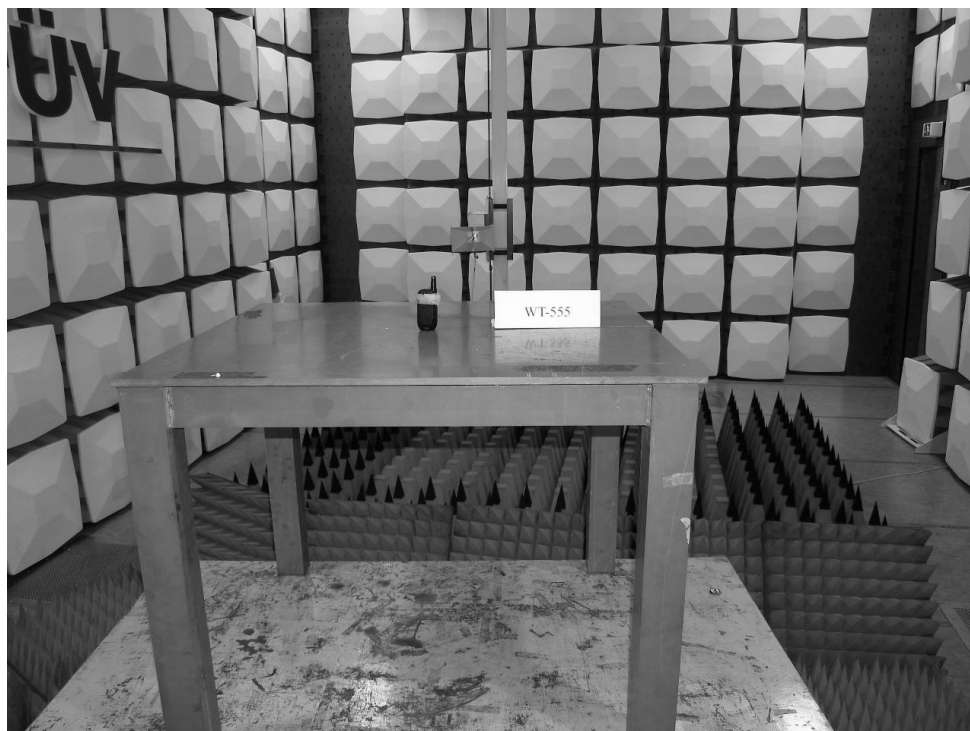
Photograph 4: Set-up for Spurious Radiation Emission Measurement above 1GHz
