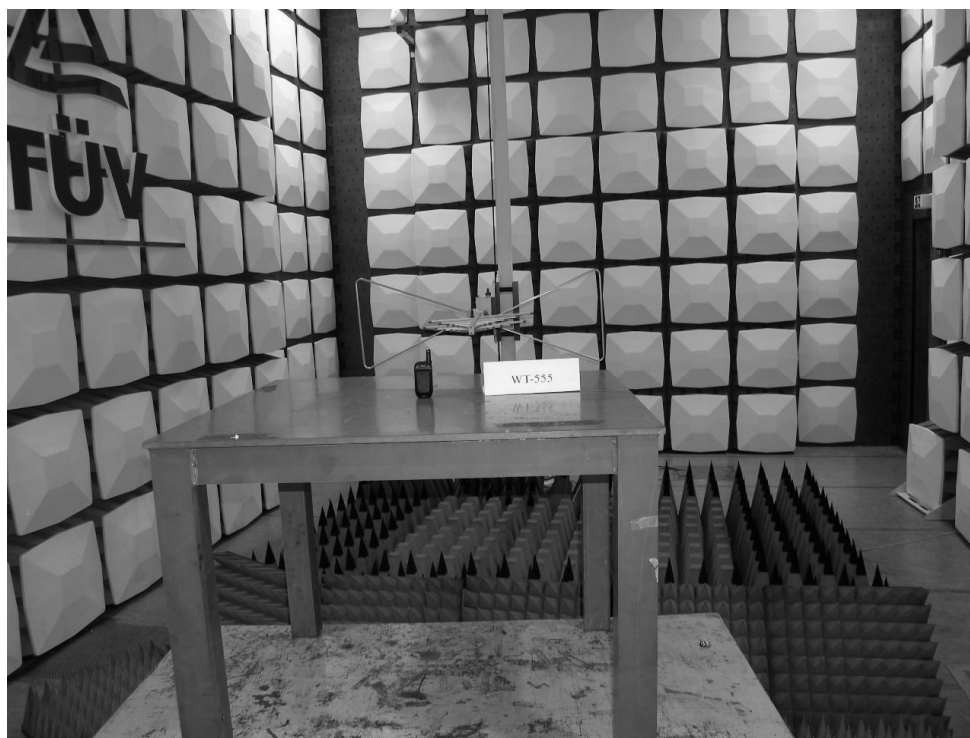
Photograph 3: Set-up for Spurious Radiation Emission Measurement below 1GHz
