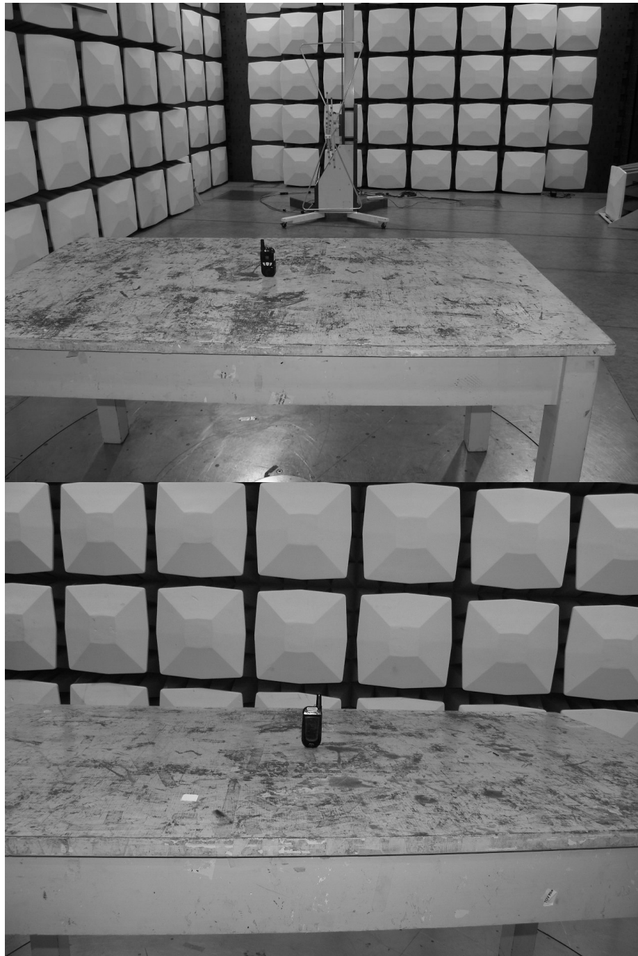
Photograph 1: Set-up for Radiation Measurement Below 1GHz
