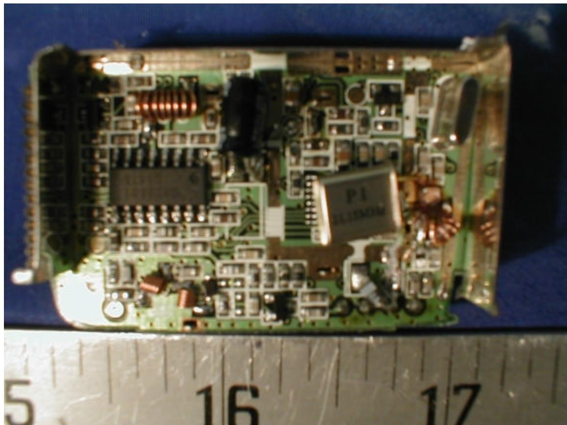
**EUT – Transmitter Solder View**
