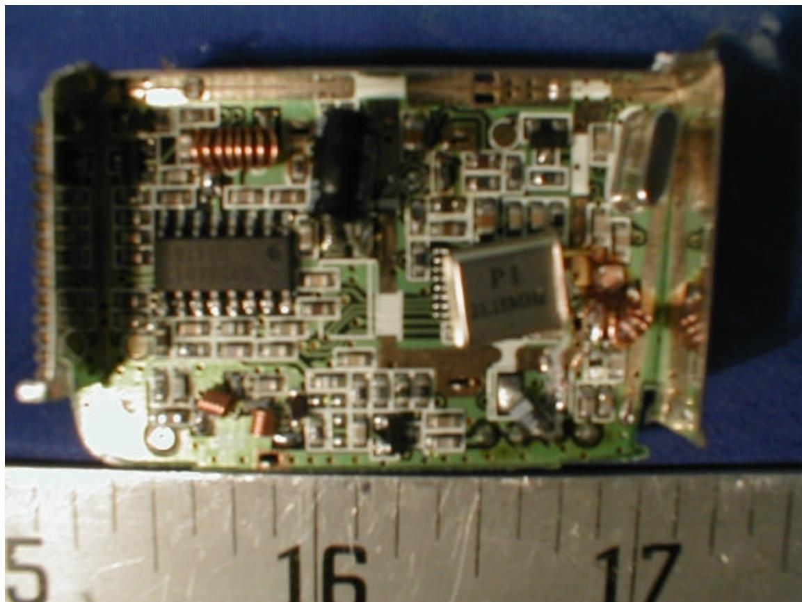
**EUT – Transmitter Solder View**
