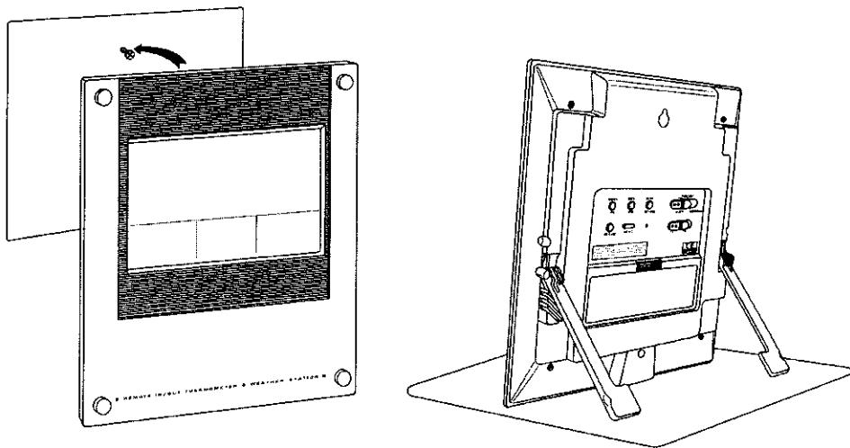
The remote unit comes with a wall mount holder which can hold the unit on wall, or just place it on a flat surface.
