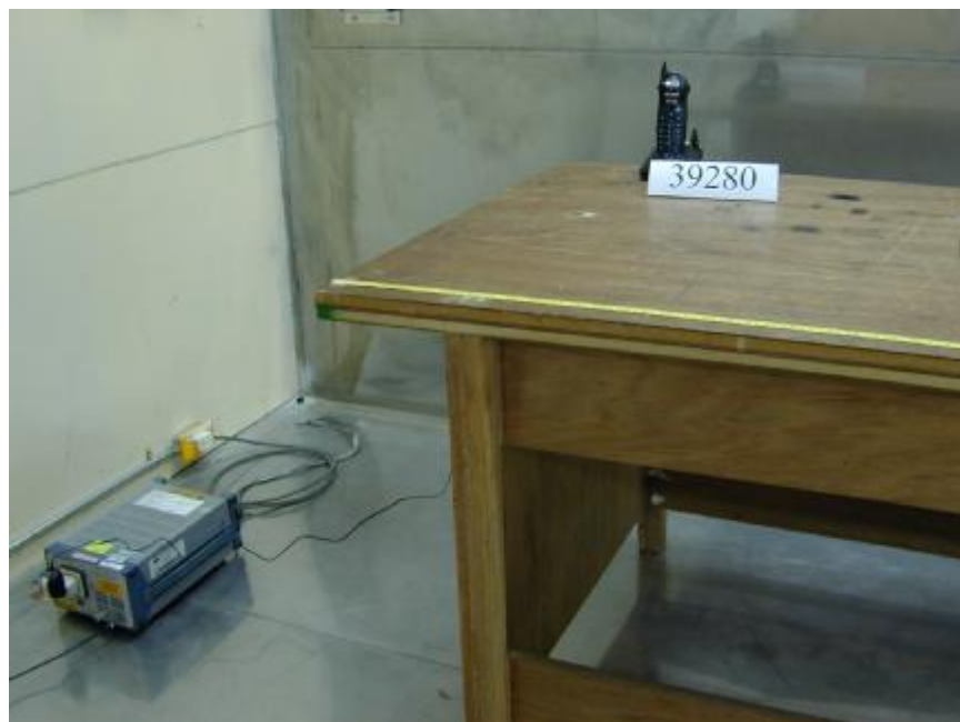
Photo 2: Conducted Emission Test Set-up
