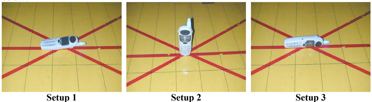
After verifying three axes, the worst case was occurred at setup 3 configuration. The final test was executed under this configuration and recorded in this report.
