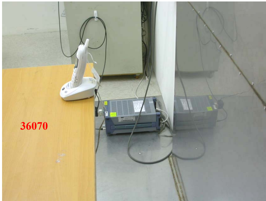
Photo 2: Conducted Emission Test Set-up photo
