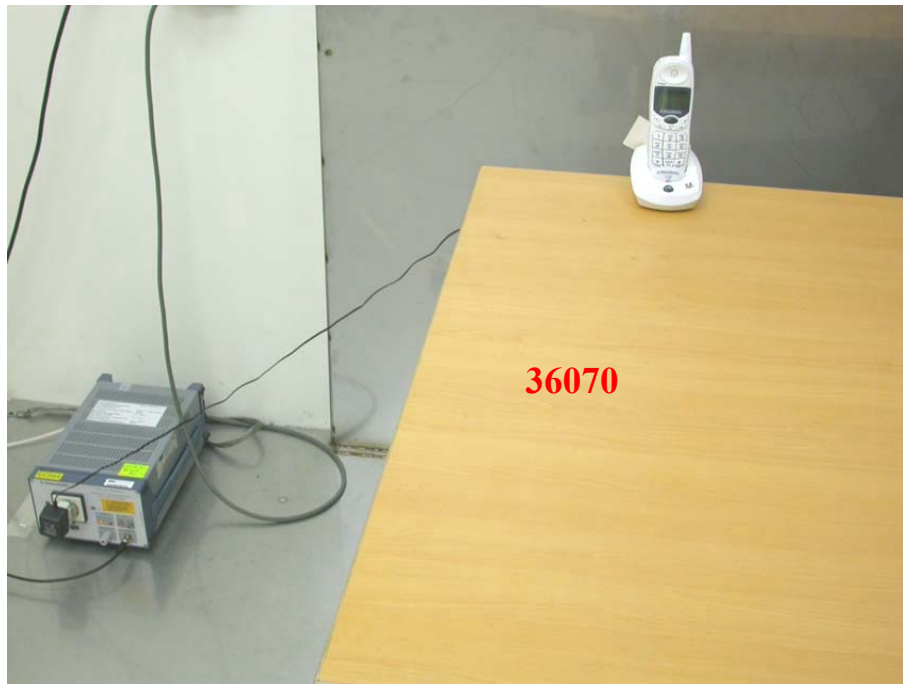
Photo 1: Conducted Emission Test Set-up photo
