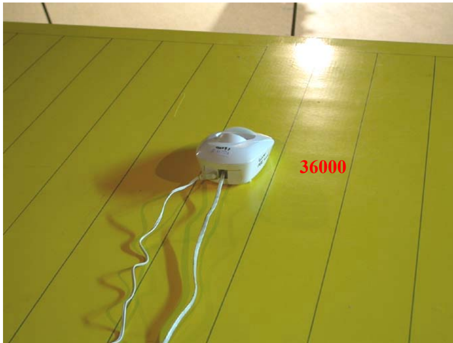
Photo 2: Radiated Emission Test Set-up photo (Base)
