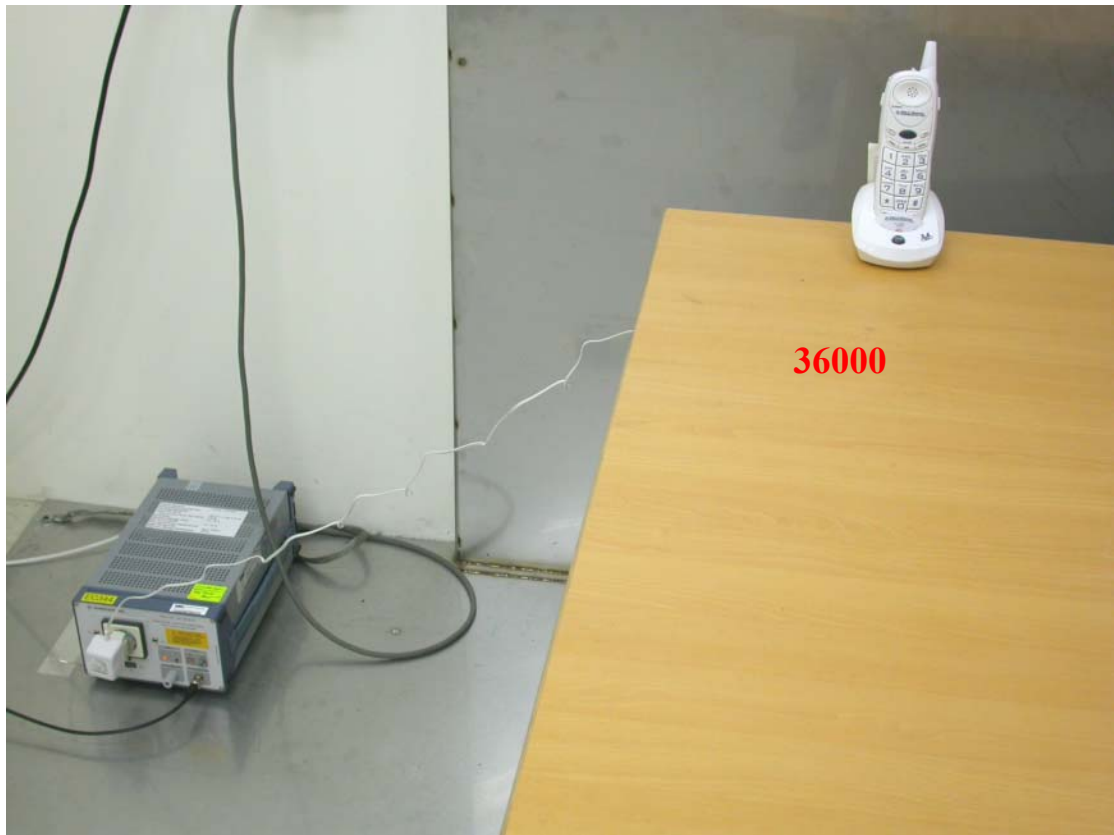
Photo 1: Conducted Emission Test Set-up photo
