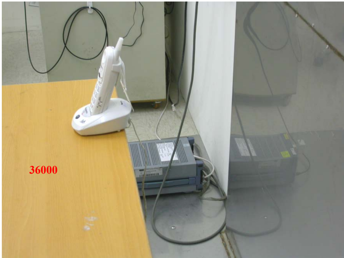
Photo 2: Conducted Emission Test Set-up photo
