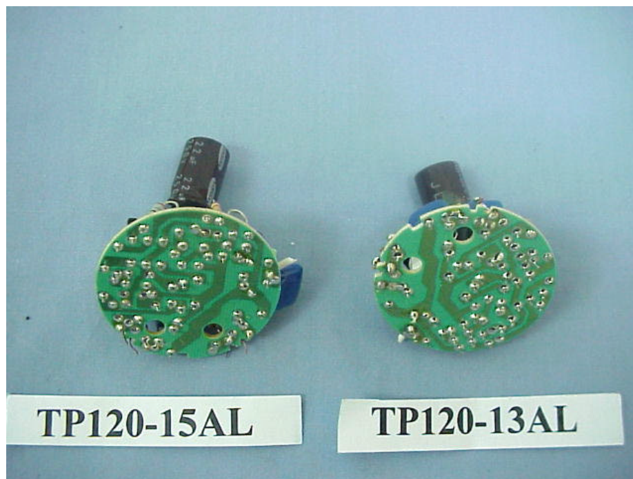
Figure 12. Compact Fluorescent Lamp (M/N: TP120-AL Series) Main Board (Soldered Side)
