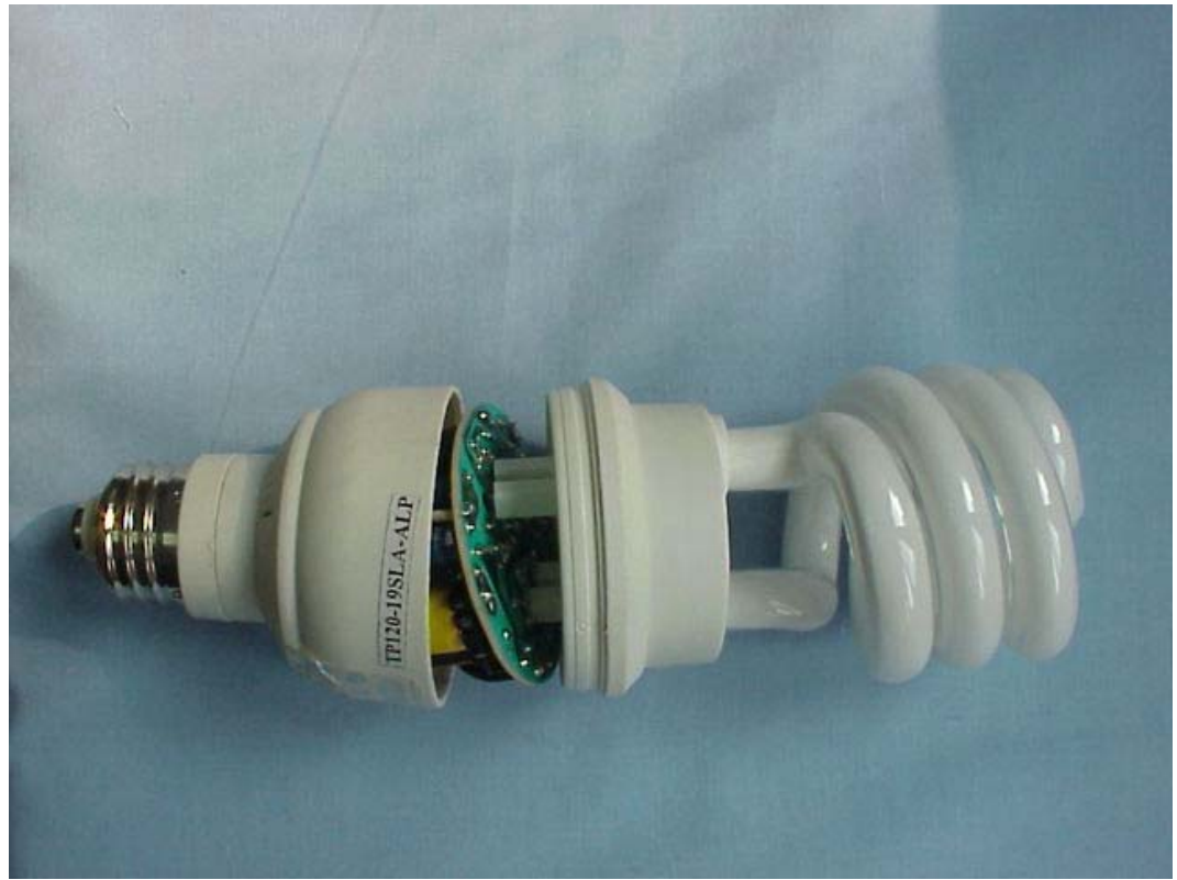
FIGURE 7 ENERGY SAVING LAMP (M/N: TP120-19SLA-ALP) COVER REMOVED
