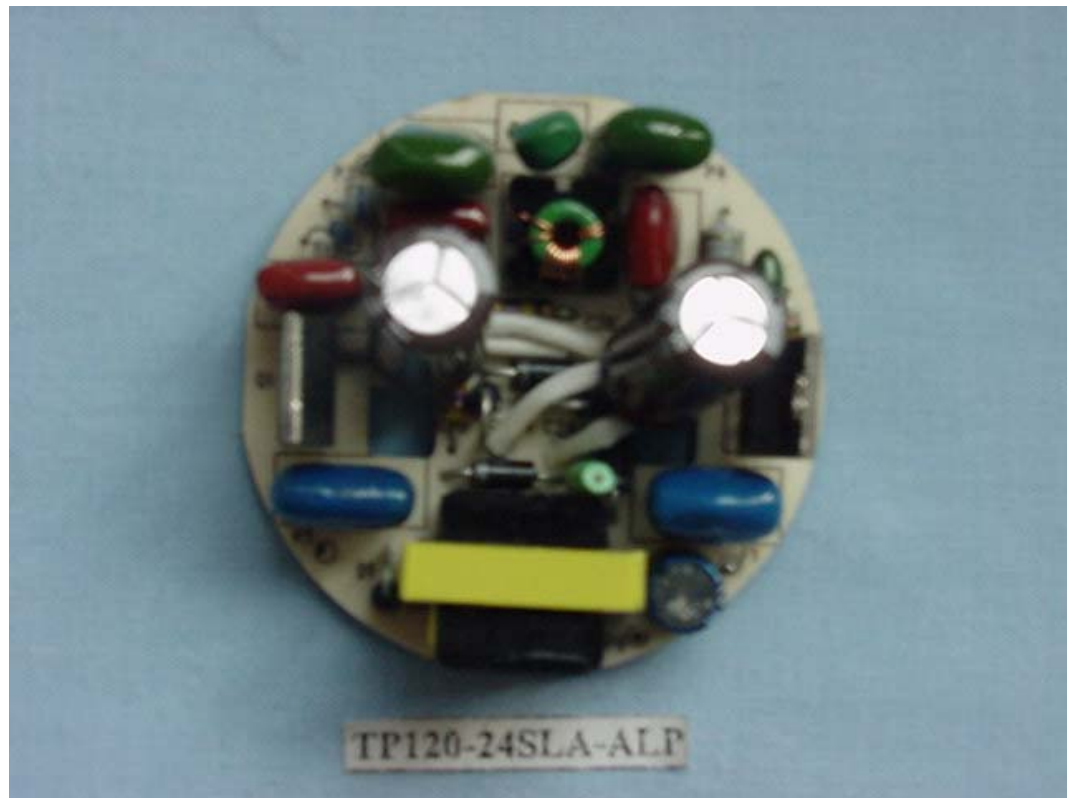
FIGURE 11 ENERGY SAVING LAMP (M/N: TP120-24SLA-ALP) MAIN BOARD (COMPONENT SIDE)
