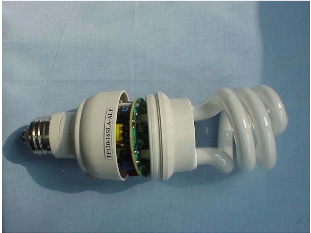
FIGURE 4 ENERGY SAVING LAMP (M/N: TP120-16SLA-ALP) COVER REMOVED
