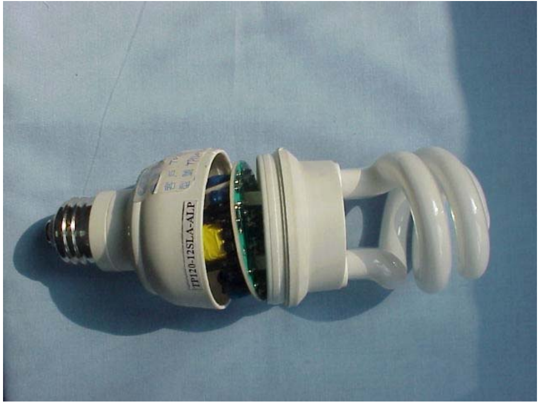
FIGURE 1 ENERGY SAVING LAMP (M/N: TP120-12SLA-ALP) COVER REMOVED
