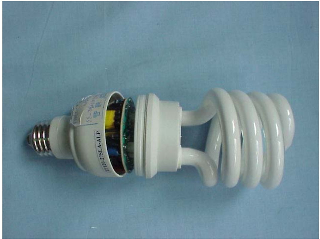
FIGURE 13 ENERGY SAVING LAMP (M/N: TP120-27SLA-ALP) COVER REMOVED
