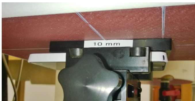
Photo of the device positioned for WR mode measurement –back facing phantom. The spacer was removed before the start of the measurements.
