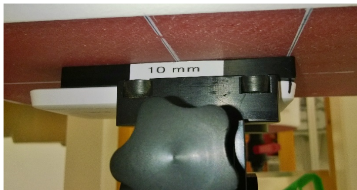
Photo of the device positioned for WR mode measurement – display facing phantom. The spacer was removed before the start of the measurements.
