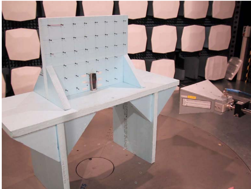
Picture 3: Radiated spurious emission measurement set-up for above 3 GHz measurements, EUT in vertical orientation
