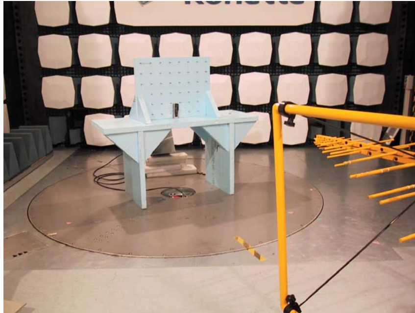
Picture 2: Radiated spurious emission measurement set-up for below 3 GHz measurements, EUT in vertical orientation
