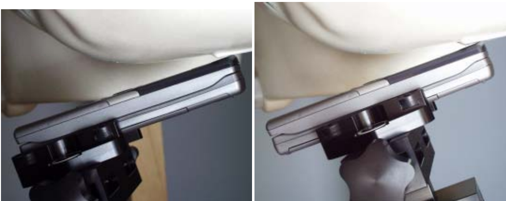
Photo of the device in “tilt” position, for GSM testing on the left and for WLAN on the right
