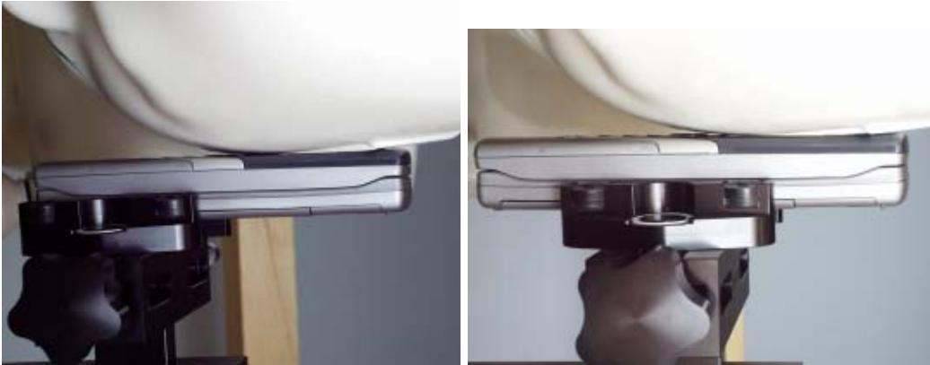
Photo of the device in “cheek” position, for GSM testing on the left and for WLAN on the right
