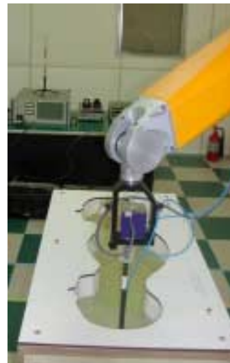
Figure 4. Photograph of the probe and the Phantom
