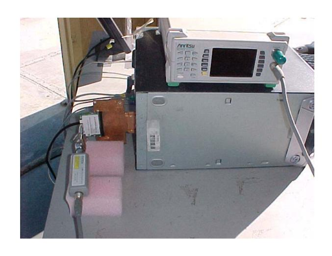
Maximum Peak Output Power Measurement Setup
