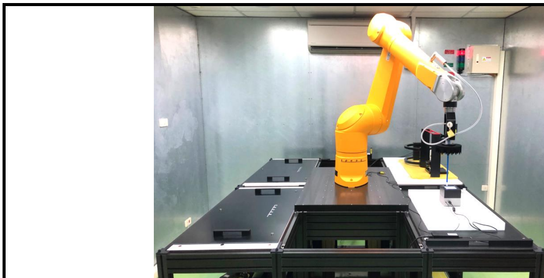
Fig-3.2 SPEAG DASY6 System
