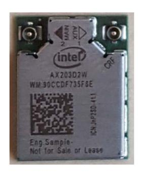
Due to the small size of the module 12mm x 16mm the FCC and ISED IDs will be published in the Information Guide.
