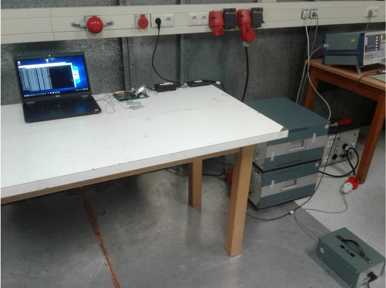
Photo 5: Photograph conducted emissions 0.15-30 MHz
