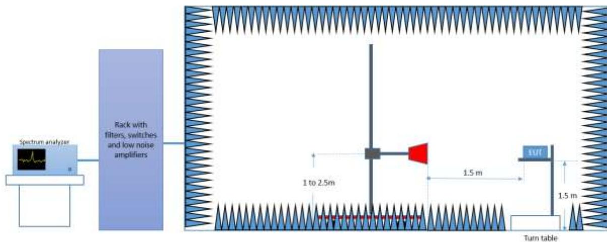
Test Results**30 MHz – 40 GHz, 802.11a, 6Mbps, Chain A Div1****Radiated Spurious – CH100**
