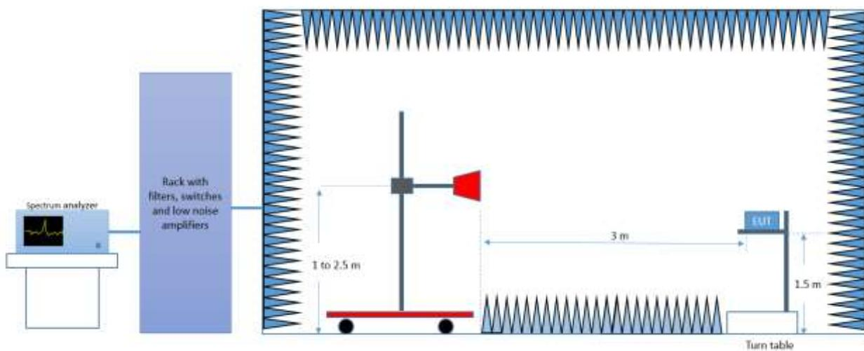
*Radiated Setup 6.4 GHz - 18 GHz*
