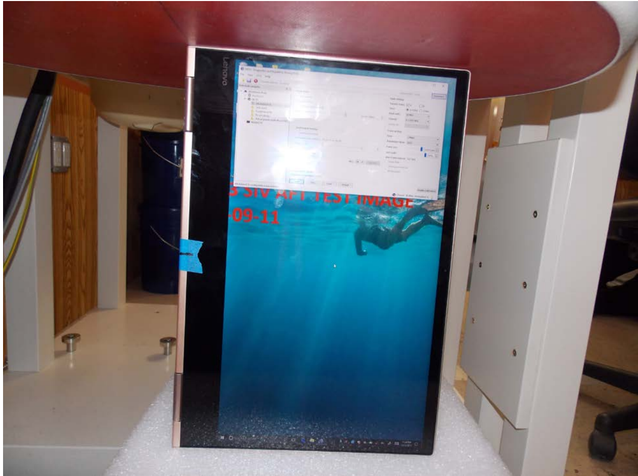
Test Position Left 0 mm Gap
