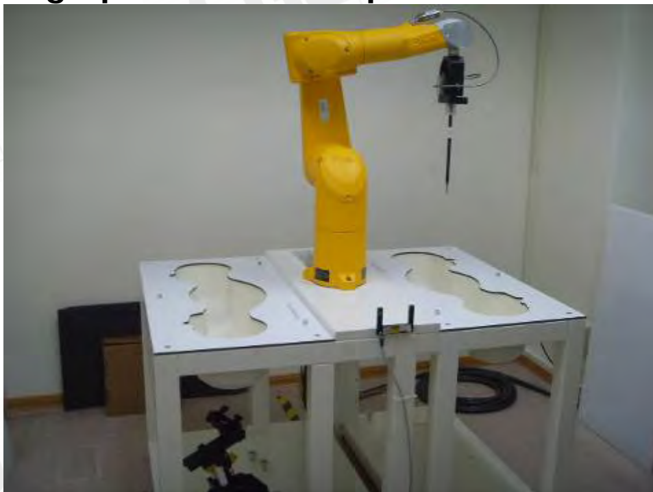
Fig.1 Photograph of the SAR measurement System
