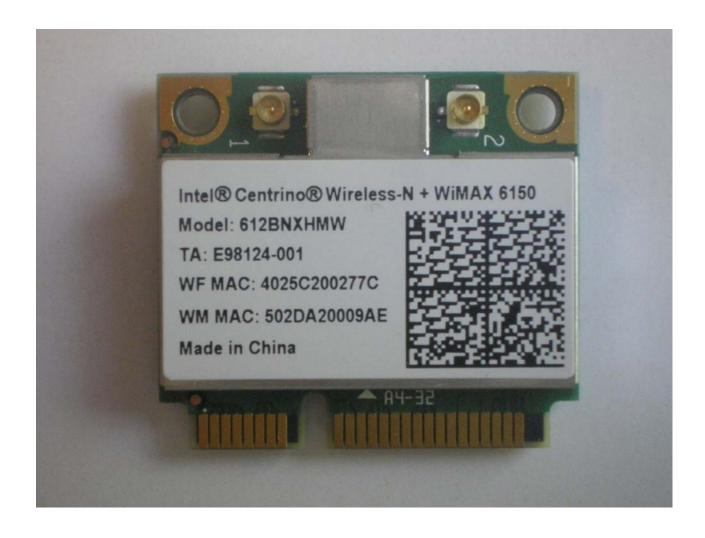
Photo showing label placement on half-mini card.
