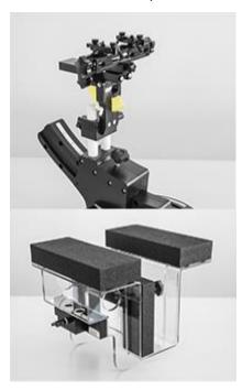
would produce a SAR uncertainty of 20%. Accurate device positioning is therefore crucial for accurate and repeatable measurements. The positions in which the devices must be measured are defined by the standards.
